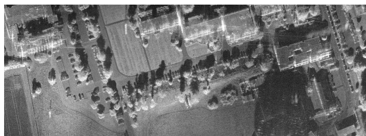
SAR image of the compound of Fraunhofer FHR measured with MIRANDA-94 with 94 GHz operational frequency and 2 GHz bandwidth. The resulting image resolution is 7.5 cm.
